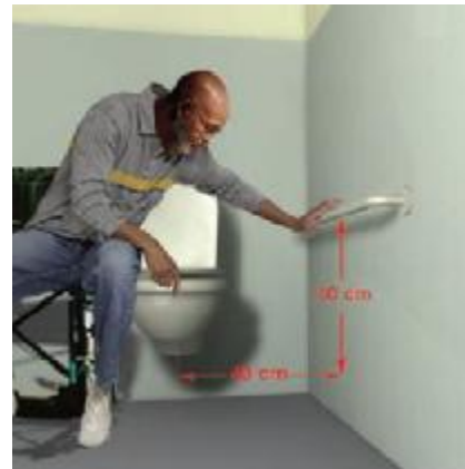
Figure 12: Grab bar distance from wall and toilet Source: Guidelines for the Planning of Houses for Senior Citizens, 2007
