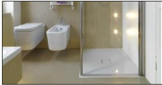
Figure 4: shower area has a glass partition to prevent water from going outside and may lead to falling down. Source: Guidelines for the Planning of Houses for Senior
