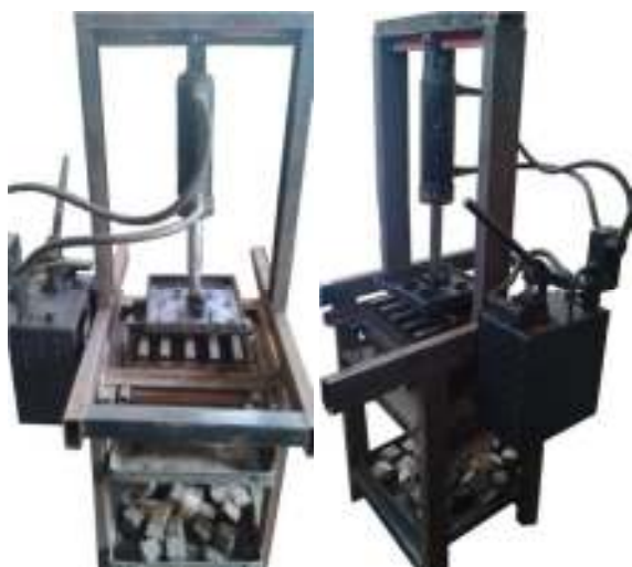
Fig. 1. Photo for the used mechanical compressor.
