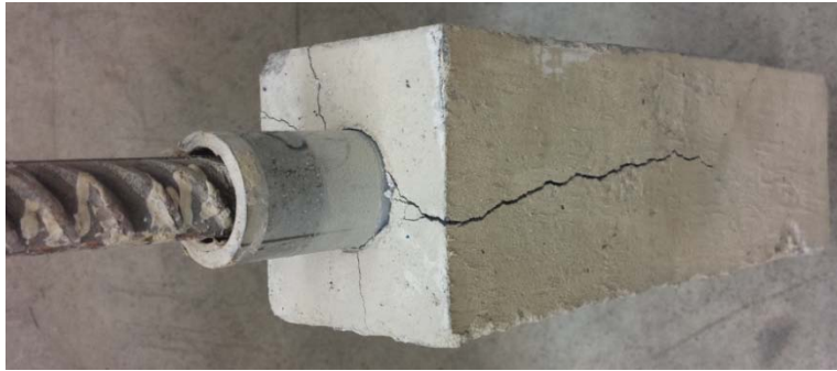
Fig. 2 Typical bond splitting cracks at failure (example sample: 20M30B-1)
