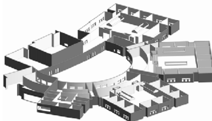
Figure 2 The school's wall assemblies
