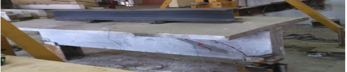
Beam (f) flange width equal 900 mm-splitting failure
