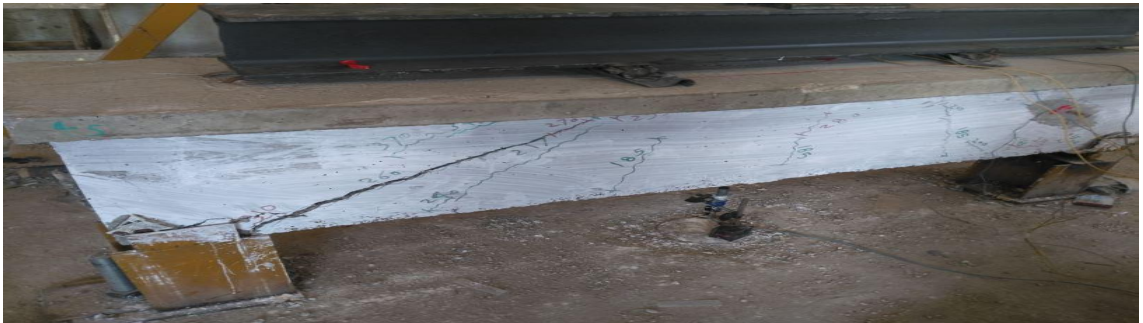
Beam (c) flange width equal 450 mm-splitting failure
