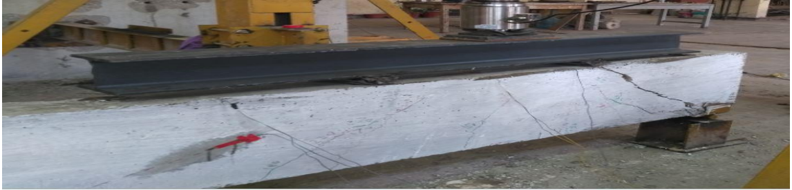
Beam (a) R- section-diagonal crushing failure
