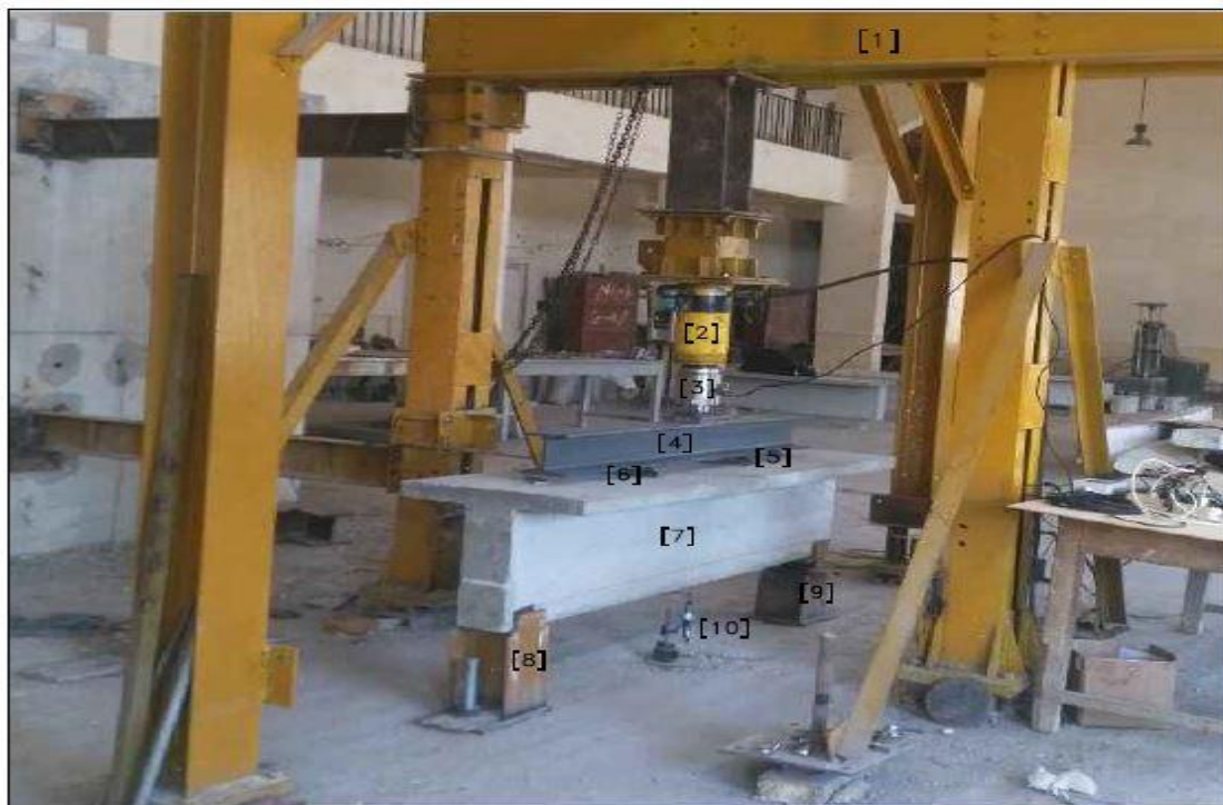
Figure (2): Test setup and system of loading.
