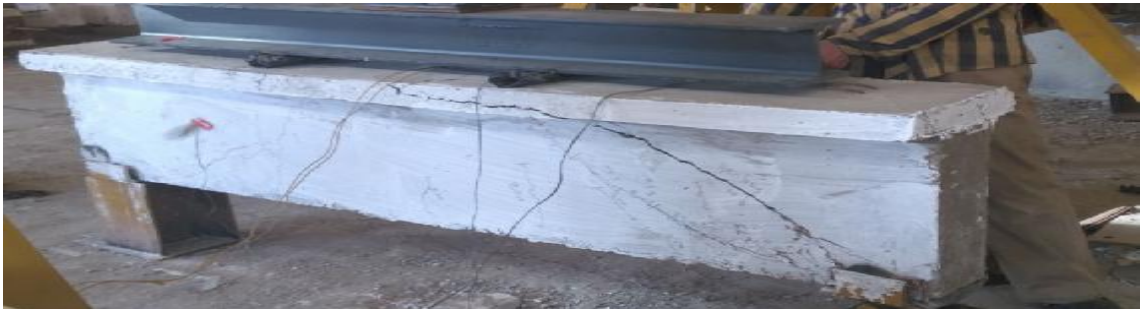
Beam (b) flange width equal 300 mm- diagonal crushing failure
