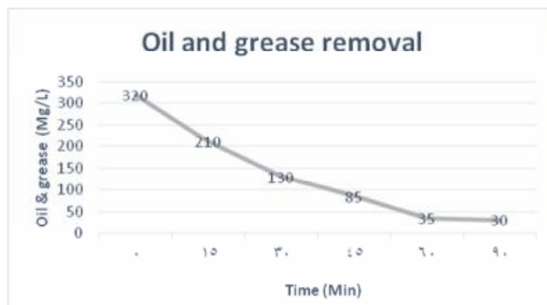
Figure (3.2) Oil and grease removal curve during different time intervals
