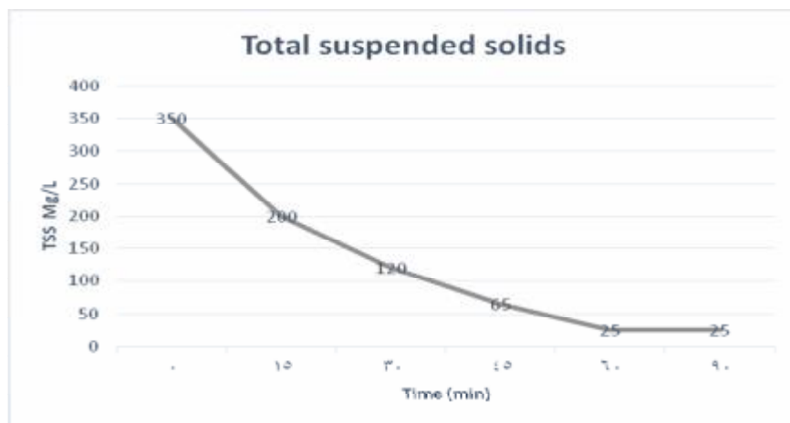
Figure (3.1) TSS removal curve during different time intervals
