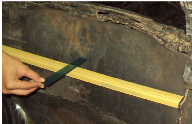
Fig. 2: Effect of 150 kg of TNT at a distance of 3m on 7mm ArmoX-500 plate
