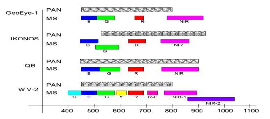
Figure 1 comparison between spectral band coverage of WV-2, QB, IKONOS and GeoEye-1
