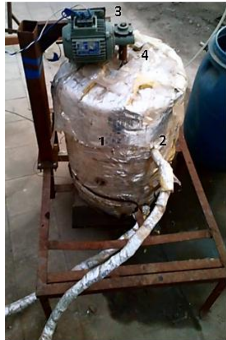
Treatment digester Photography picture
