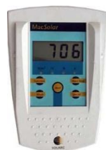
Fig. 12. Solar radiation meter model MAC SOLAR SLM018C-E, Germany
