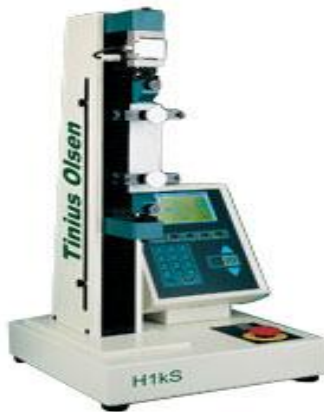
Fig. 7. Tinius Olsen bench top universal testing machine (UTM)
