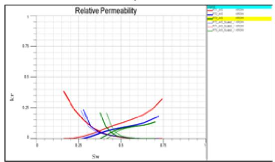
Figure 9 Oil-water relative permeability - end point scaling for different rock.
