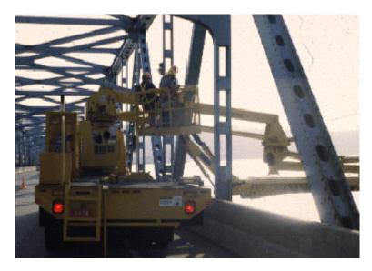
Figure 1. Mobile man-lift device.
