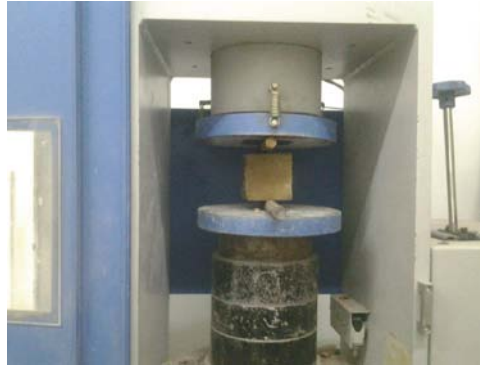
Figure 5 Indirect tension test for polyester mortar cubes.
