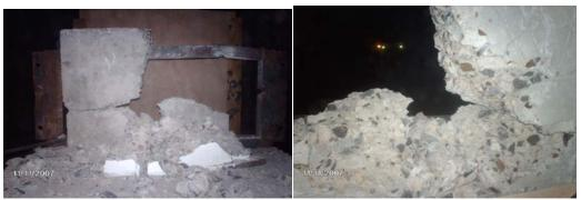
Damage in Front Face of plain concrete slab Damage in rear Face of plain concrete slab
