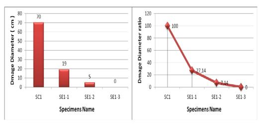
Figure (10): Effect of using ferrocement on damage in rear face
