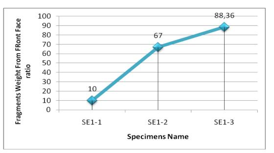
*Figure (11): Effect of using ferrocement on fragments weight in front face (cont.)*
