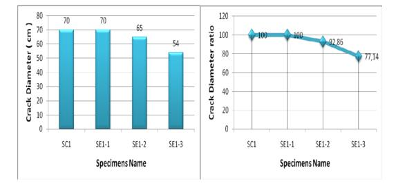
Figure (7): Effect of using ferrocement on cracks in front face
