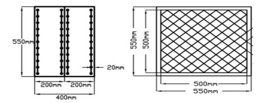
Figure (4): Dimensions and details of the specimen
