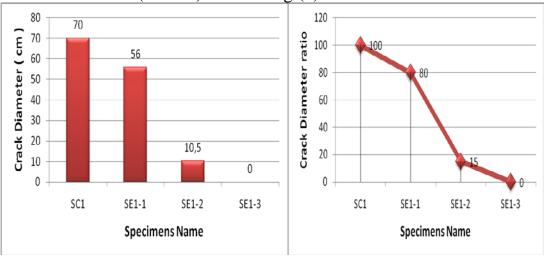
Figure (8): Effect of using ferrocement on cracks in rear face
