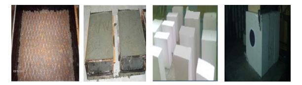
Figure (1): square plain concrete and ferrocement specimens
