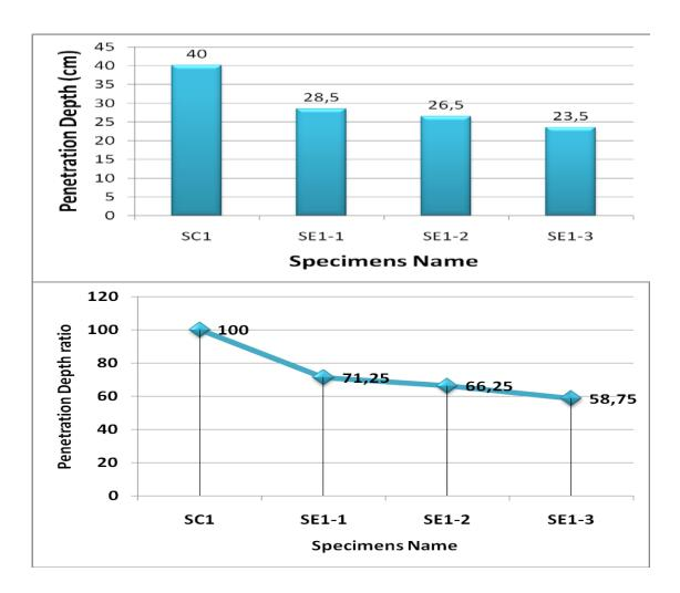
Figure (6): Effect of using ferrocement on penetration depth
