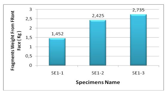
*Figure (11): Effect of using ferrocement on fragments weight in front face*
