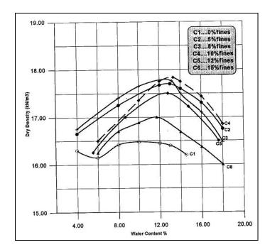
Figure (3): Effect of fines content on the moisture-density relation
