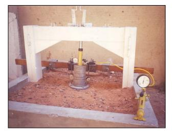
Figure (2): Plate loading test setup
