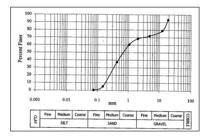
Figure (1): Grain size distribution of the tested soil
