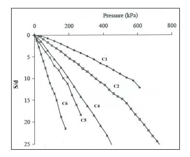
Figure (6): Effect of fines content on bearing capacity
