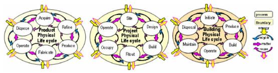
Fig. 8: Flow Diagrams of Products & Building Physical Life Cycle Phases, Source: [33]
