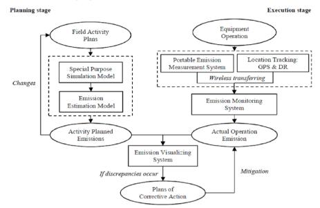
Fig. 5: Emission Management Framework for Construction Processes, Source: [20]
