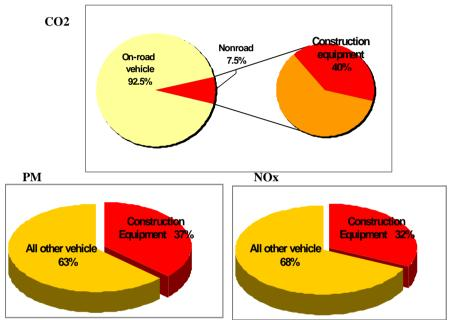
Fig. 4: HAPs Emissions of Construction Equipment Related to Vehicle, Source: [20]
