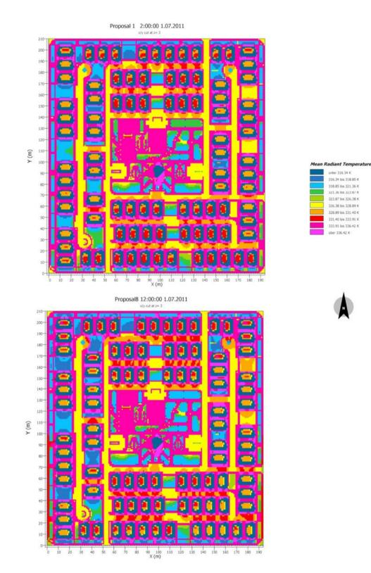
Figure (9): Tmrt mapping for BCPD, P1PD and P2PD respectively, at 12.00 LST.
