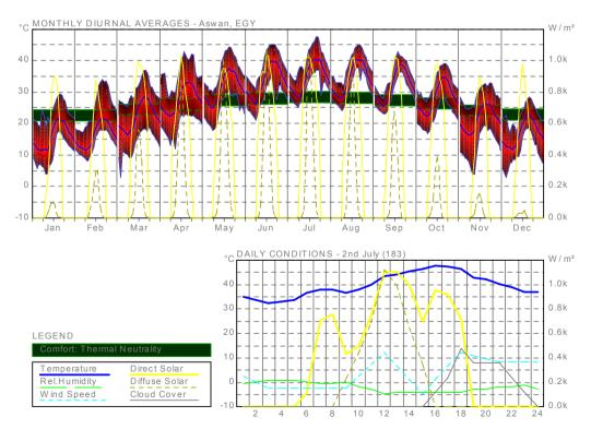
**Figure (3):** Meteorological measurements at WMO weather station no. 624140 of Aswan corresponding to the extreme hot summer day analyzed by ECOTECT 2010.
