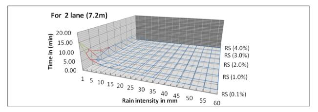
Figure (11): Shows the time of rains remains on the road surface consist of 2 lanes with manning coefficient 0.016 with different side slope (RS) and rain intensity.
