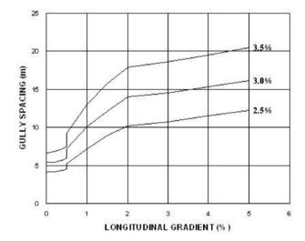
Figure (1) the effect of longitudinal gradient on gully spacing
