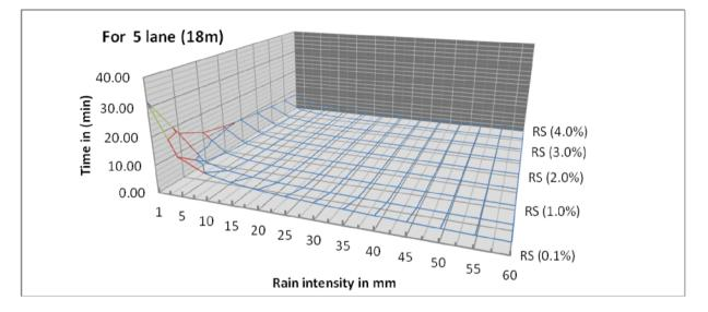
Figure (14): Shows the time of rains remains on the road surface consist of 5 lanes with manning coefficient 0.016 with different side slope (RS) and rain intensity.
