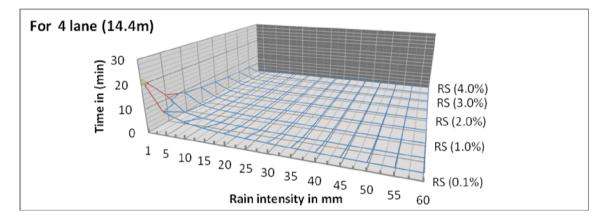
Figure (8): Shows the time of rains remains on the road surface consist of 4 lanes with manning coefficient 0.013 with different side slope (RS) and rain intensity.
