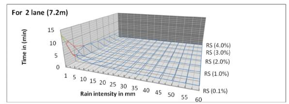
manning coefficient 0.013 with different Cross slope (RS) and rain intensity.
