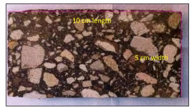
Figure (3) specimen dimension
