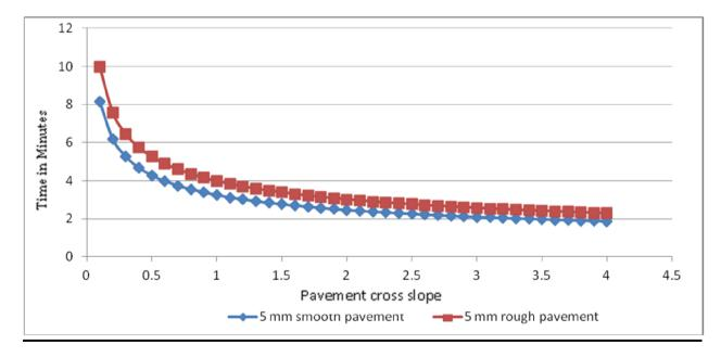
Figure (21) comparison between smooth and rough pavement drainage
