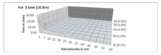
Figure (12): Shows the time of rains remains on the road surface consist of 3 lanes with manning coefficient 0.016 with different side slope (RS) and rain intensity.
