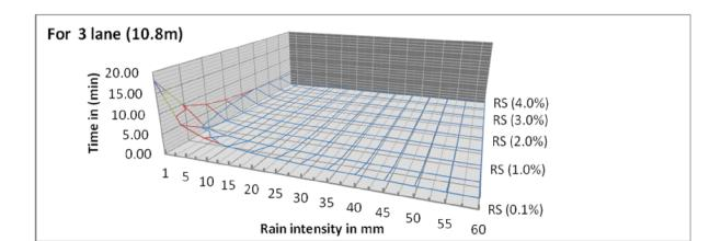
manning coefficient 0.013 with different side slope (RS) and rain intensity.
