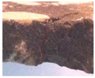
Figure (17) hair cracks appears in the x-ray picture
