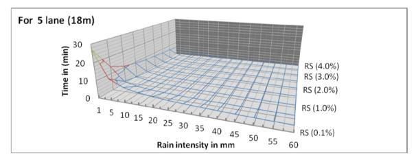
Figure (9): Shows the time of rains remains on the road surface consist of 5 lanes with manning coefficient 0.013 with different side slope (RS) and rain intensity.
