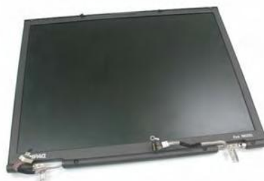
Figure (11): LCD Pane, as example for a transmissive display
