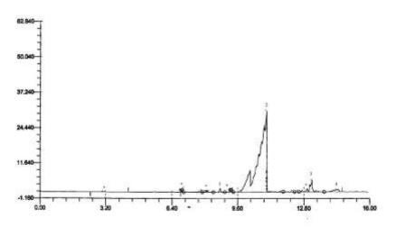
Figure 3. GLC chromatogram of anise oil (Phosphorene +NPK (3).
