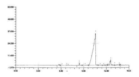
Figure 2. GLC chromatogram of anise oil (Phosphorene).
