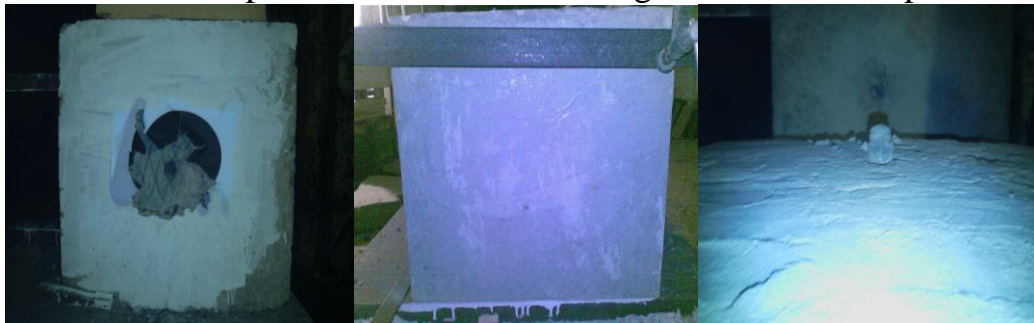
Damage in Front Face of ferrocement slab Damage in rear Face of ferrocement slab projectile stopped inside the panel
