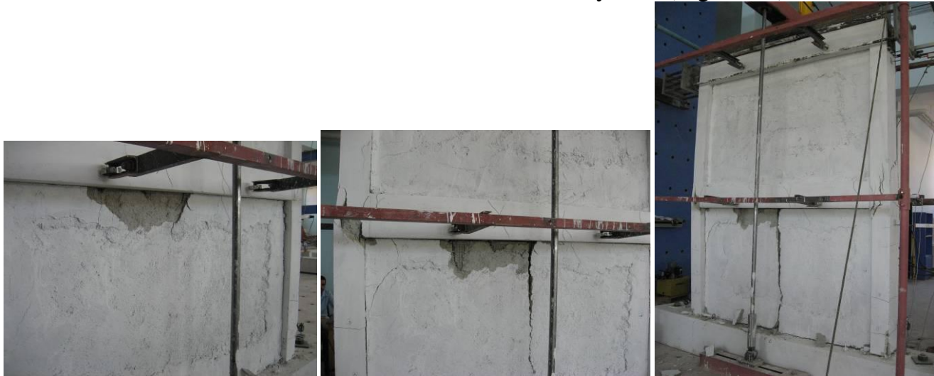
Figure (10) Failure mode of the specimen SP3
