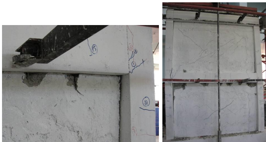
Figure (11) Failure mode of the specimen SP4
