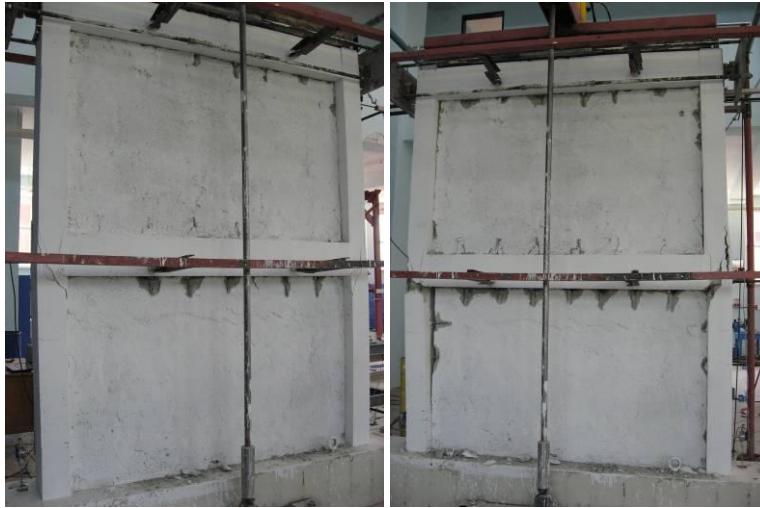
Figure (9) Failure mode of the specimen SP2
