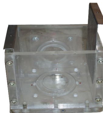
Fig. 1a, Cross section view in the mold used for ultrasonic velocity and electrical resistivity measurements. Fig. 1b, Photograph of the mold used for ultrasonic velocity and electrical resistivity measurements.
