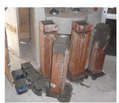
Fig.3 Concrete jacket after casting
