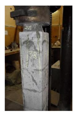
Fig.8 Jacket failure of group (C)
