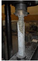
Fig.5 Original column failure
