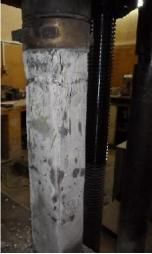
Fig.6 Jacket failure of group (A)
