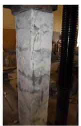
Fig.7 Jacket failure of group (B)
