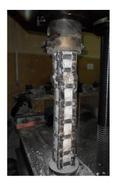
Fig.11 Jacket failure of group (E)
