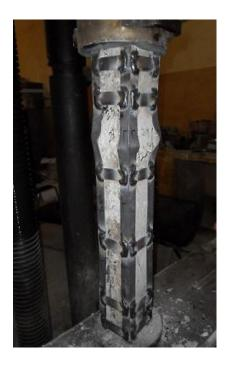
Fig.9 Jacket failure of group (D)
