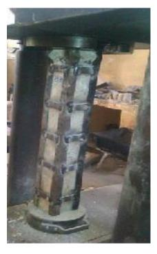
Fig.10 Jacket failure of group (D'')
