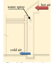
Figure 8 : Evaporative cooling system proposal
