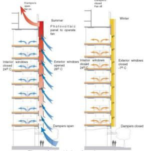
Figure 18 : Double interfaces System(17).
