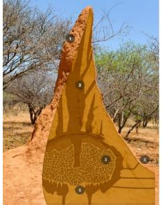
Figure 19: Systems of cooling by natural carriage ducts inside the Termite nest
