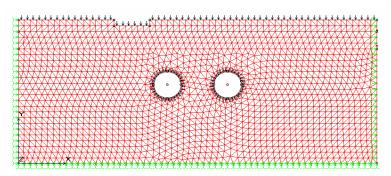
Fig. 4: 2-D finite element model of tunnel (case history- side by side)
