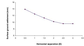
Fig. 8: Calculated settlement at ground surface with different horizontal separations (new tunnel running side-by-side old tunnel)
