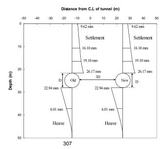
Fig. 7: Vertical displacement at different levels along centerline of twin tunnel with three-diameter horizontal separation
