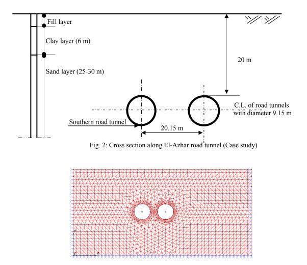
Fig. 3: 2-D finite element model of tunnel (new tunnel running side by side to existing tunnel)
