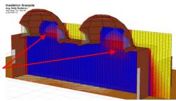
Fig. 8: Thermal infiltration through windows
