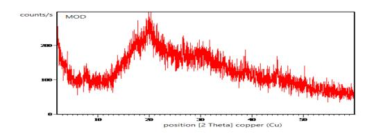
Fig. 1. X-ray diffraction of modified chitosan.
