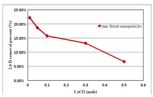
Fig. 9. Effect of ions strength on zinc ferrite nanoparticles photocatalytic degradation. Using a dose of 0.3g/50ml and initial 2,4-D concentration 10mg L-1
