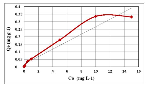
Fig. 6. Effect of adsorption capacity of Zinc ferrite nanoparticles against initial concentration of 2,4-D at Zinc ferrite nanoparticles dosage 0.3g/50ml
