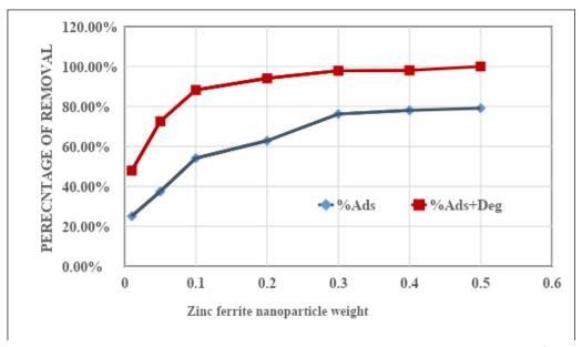
Fig. 5. Effect of zinc ferrite nanoparticles weight on the removal %. 2,4-D initial concentration 5 μg L<sup>-1</sup>and contact time 15 min.
