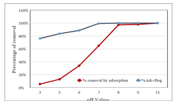
Fig. 4. Effect of pH on the removal %. Initial 2,4-D concentration 1 µg L-1, zinc ferrite nanoparticles dosage 0.2 g and contact time 15min.
