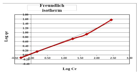
Fig. 11. Freundlich adsorption isotherm of 2,4-D on Zinc ferrite nanoparticles.
