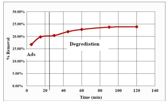
Fig. 7. Effect of contact time. Zinc ferrite nanoparticles dose 0.3g/50ml and 2,4-D initial concentration 10mg L-1
