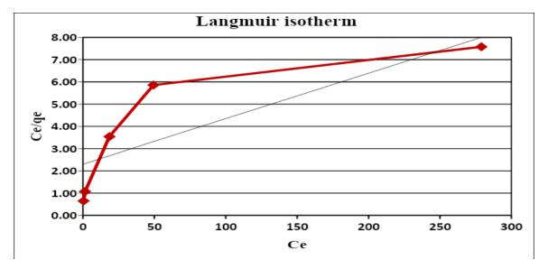
Fig. 12. Langumuir adsorption isotherm of 2,4-D on Zinc ferrite nanoparticles
