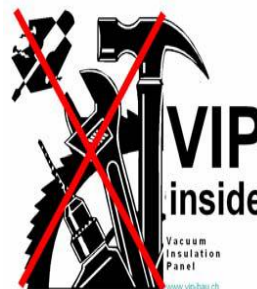
Figure (6): Draft sketch for an adhesive warning label to mark VIP panels and building components containing VIP
