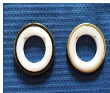
Fig.3: Molds for preparing cemented ceramic veneers samples
