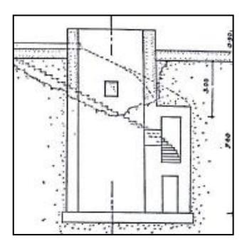
Fig.13 Nilometer in the form of a spiral staircase surrounds a circular well at temple of Mandaulis at Kalabsha
