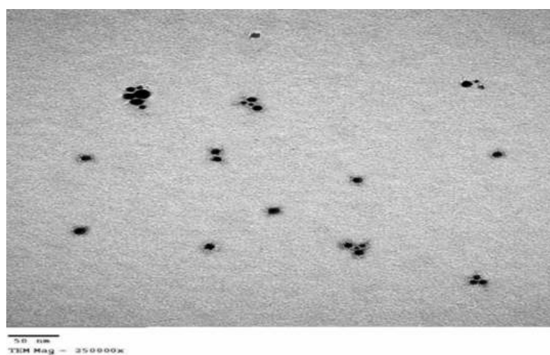
Fig. 12. TEM electron micrograph of AgNPs produced by Bacillus subtilis ssp spizizenii MT5
