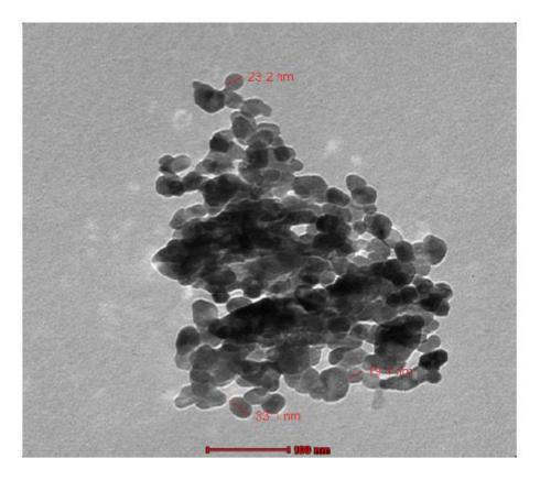
Fig. 5. TEM image of chemically synthesized ZnO NPs
