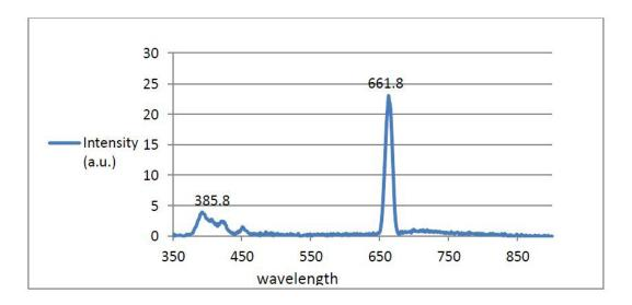
Fig. 8. photoluminescence spectrum of chemically synthesized ZnO NPs.
