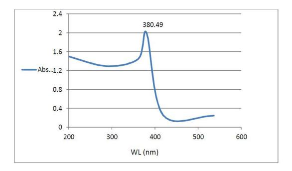
Fig. 7. UV-vis spectrum of chemically synthesized ZnO NPs.
