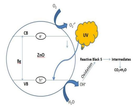
Fig. 12. Photo-induced formation mechanism of electron-hole pair in semiconductor ZnO particles with the presence of RB5 dye.
