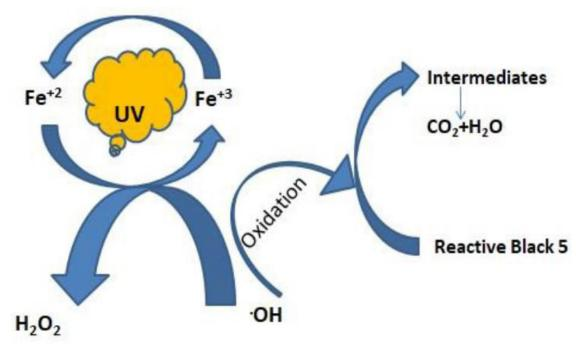
Fig. 13. Photo-Fenton oxidation mechanism for RB5 dye
