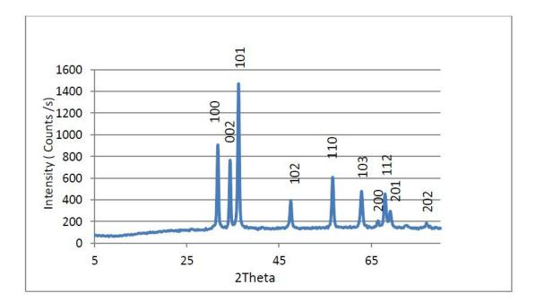
Fig.6. XRD spectra of chemically synthesized ZnO NPs
