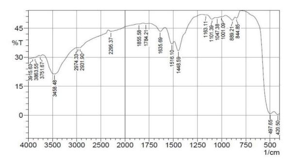
Fig.3. FTIR spectrum of chemically synthesized ZnO NPs.
