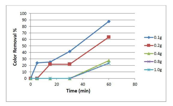
Fig. 9a. Effect of different ZnO catalyst dose on photocatalytic degradation of RB5 during the first 1h photocatalytic process at pH=7 and 1 ml of H<sub>2</sub>O<sub>2</sub> (35%).
