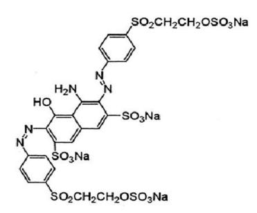
Fig.1. Chemical structure of RB5 (Molecular Formula:  $C_{26}H_{21}N_5Na_4O_{19}S_6$ ) (Molecular Weight: 991.82).  $\lambda_{Max} = 597nm$ ; C.I.20505.
