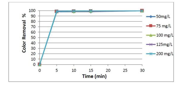
Fig. 11. Effect of initial concentrations of RB5 on the photocatalytic degradation (by using 0.1 g of FeSO<sub>4</sub>.7H<sub>2</sub>O) at pH=7 and 1 ml of H<sub>2</sub>O<sub>2</sub> (35%) under UV irradiation.
