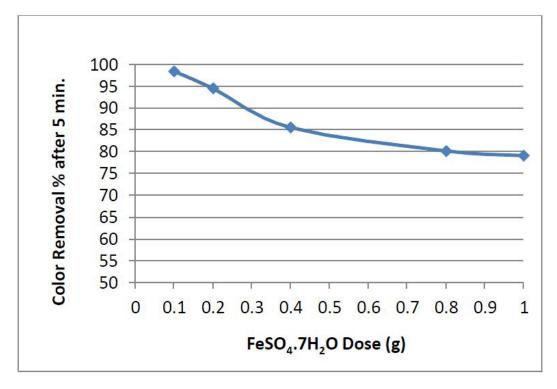
Fig. 10b. Effect of different FeSO<sub>4</sub>.7H<sub>2</sub>O catalyst dose on photocatalytic degradation of RB5 at pH=7 and 1 ml of H<sub>2</sub>O<sub>2</sub> (35%) and after the first 5 minutes.
