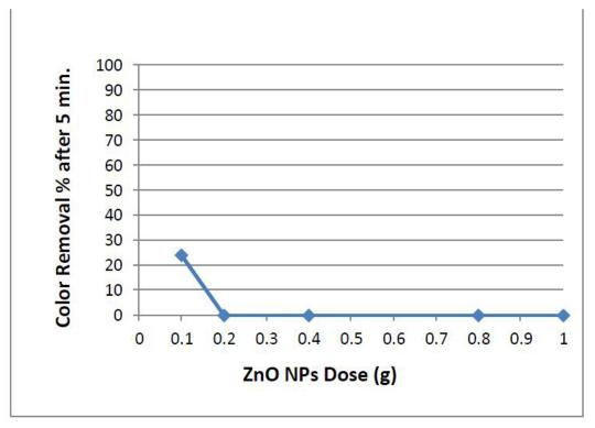
Fig. 9b. Effect of different ZnO catalyst dose on photocatalytic degradation of RB5 at pH=7 and 1 ml of H<sub>2</sub>O<sub>2</sub> (35%) after the first 5 minutes.
