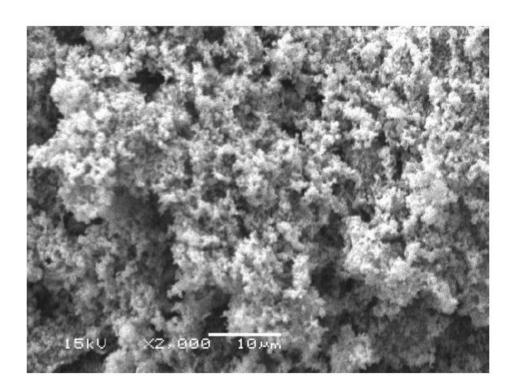
Fig. 4. SEM image of chemically synthesized ZnO NPs
