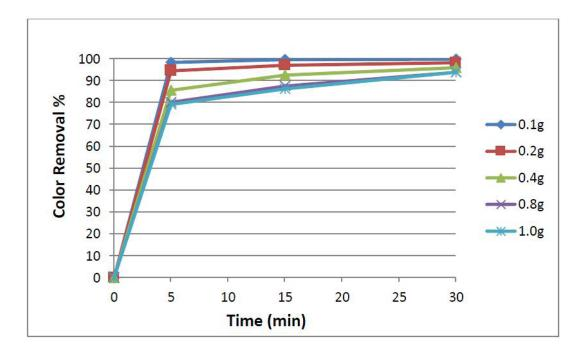
Fig. 10a. Effect of different FeSO<sub>4</sub>.7H<sub>2</sub>O catalyst dose on photocatalytic degradation of RB5 at pH=7 and 1 ml of H<sub>2</sub>O<sub>2</sub> (35%).
