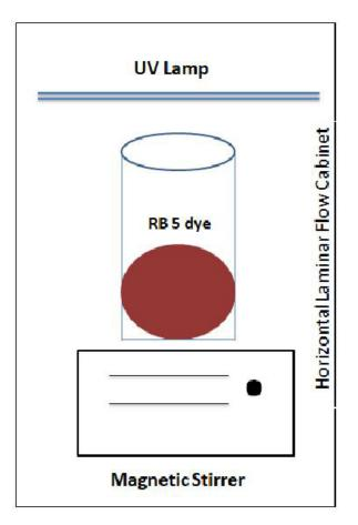
Fig.2. Schematic diagram of Photocatalytic test
