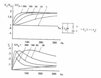
Fig. 3 Frequency behaviour of joints
