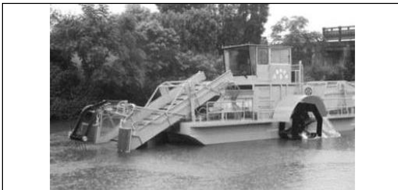
Fig. 1: A new prototype device for mechanical control water-hyacinth plants
