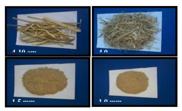
Figure 1: Raw rice straw with different particles size
