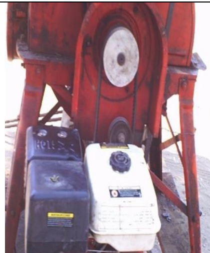
Plate 2: Diesel engine equipped with pulleys
