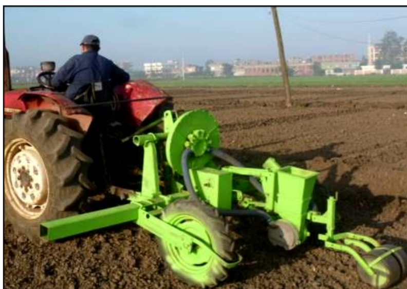
Fig. 16: Developed precision vacuum planter unit
