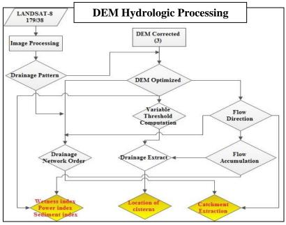
Fig. 3: Flow-chart of DEM Hydrology processing steps 875
