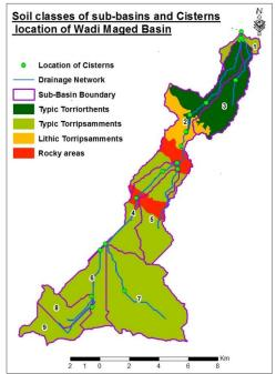
Fig. 12: Overlay of soils classes, sub-basins areas, location of cisterns and drainage network of Wadi Maged basin
