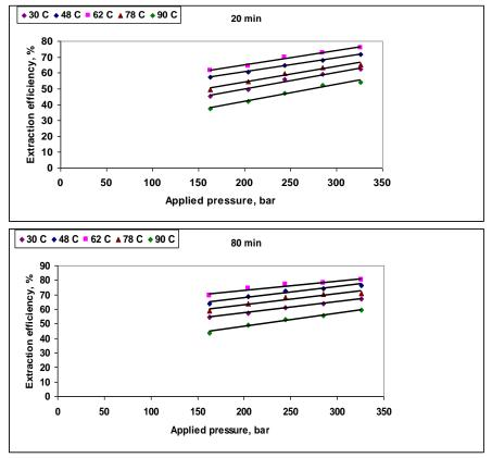
Fig. (5): Effect of applied pressure and holding time on the extraction efficiency of canola seeds heated at different levels of heating temperature.
