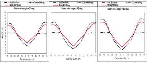
Fig. 4: Furrow profile as influenced by share rake angle and wing shape for wing angle of 45°
