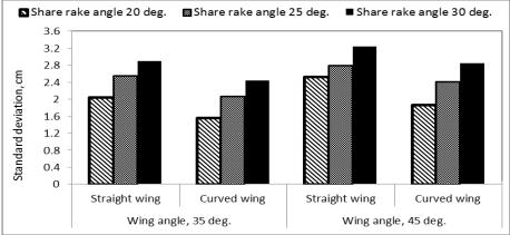
Fig.5: Effect of share rake angle, wing angle and wing shape on standard deviation of seeds scattering, cm
