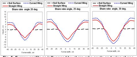
Fig. 5: Furrow profile as influenced by share rake angle and wing shape for wing angle of 35°.
