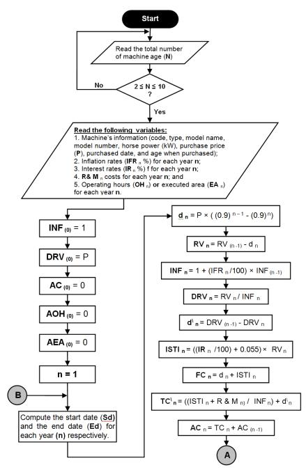
Figure (1): Flowchart of the developed computer model.
