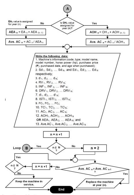
Cont. Figure (1): Flowchart of the developed computer model.
