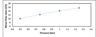
Fig. (4): Emitters flow rates vs. operating pressure (14 l/h)
