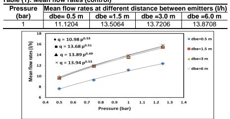
Fig. (5): Emitters flow rates vs. operating pressure before installing microtubes (control)
