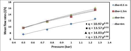
Fig. (6): Emitters flow rates vs. operating pressure after installing bypass-technique
