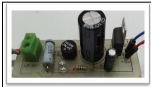
Fig 3 power supply board
