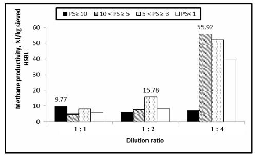
Fig. 5. Methane productivity from dry AD of sieved HSBL with respect to mass of sieved HSBL in the content of reactor
