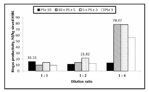
Fig. 3. Biogas productivity from dry AD of sieved HSBL with respect to mass of sieved HSBL in the content of reactor
