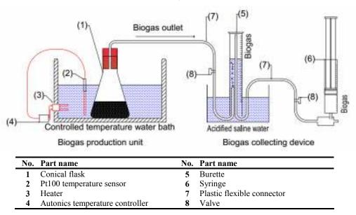
Fig. 1. Schematic diagram of laboratory scale reactor
