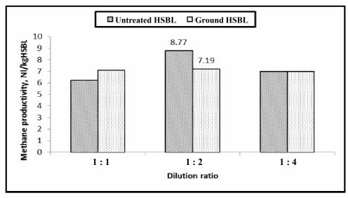
Fig. 4. Methane productivity from dry AD of untreated and ground HSBL with respect to mass of HSBL in the content of reactor
