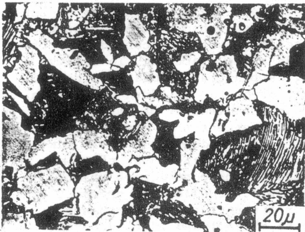
Fig.(5a) Ferritic-Pearlitic structure observed at both sides of the interface.
