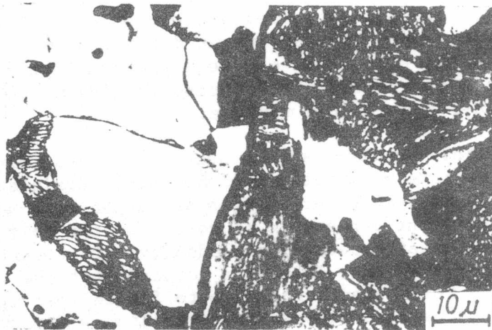
Fig.(2) Microstructure observed at the interface showing the separation between core and rim.
