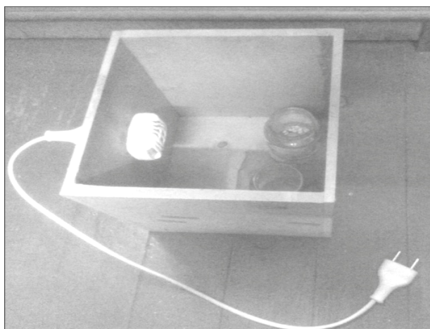
Fig 1. glass jars introduced into the fumigant chamber of approximately 6000 cm 3 with fumigant electric device
