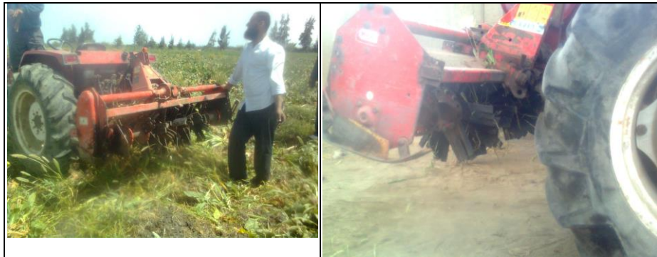
Fig. (1): The developed sugar beet topper machine.
