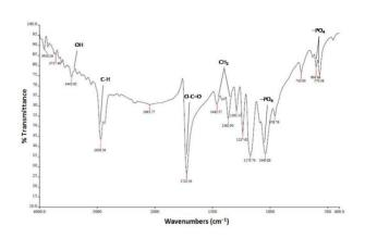
Fig. 4: ATR-FTIR spectrum of PCL/HA nano-composite samples
