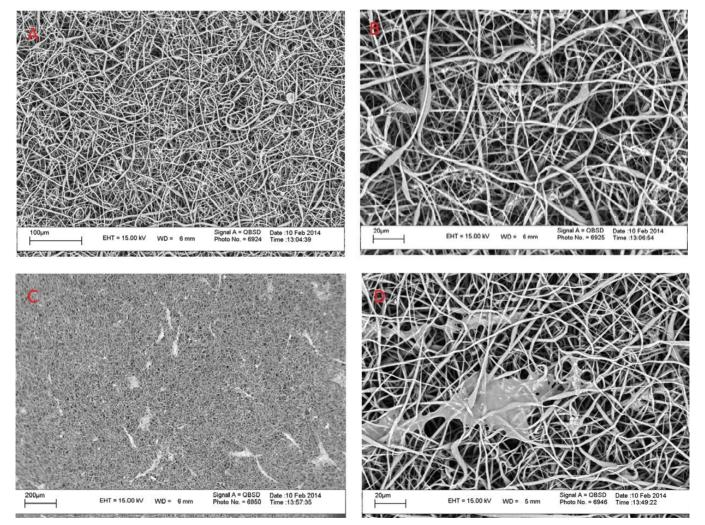
Fig. 1: SEM image of (A-B) PCL/nHA scaffold surface, scale bare is 100 and 20 µm respectively. (C) PCL/nHA scaffold, scale bare is 200 µm. (D) Cell morphology of WJ-MSCs on the scaffold (three days after seeding). Scale bar is 20µm.
