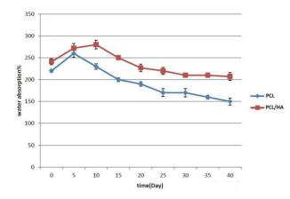
Fig. 3: Water absorption capacity of the PCL and PCL/HA scaffolds at different immersion times
