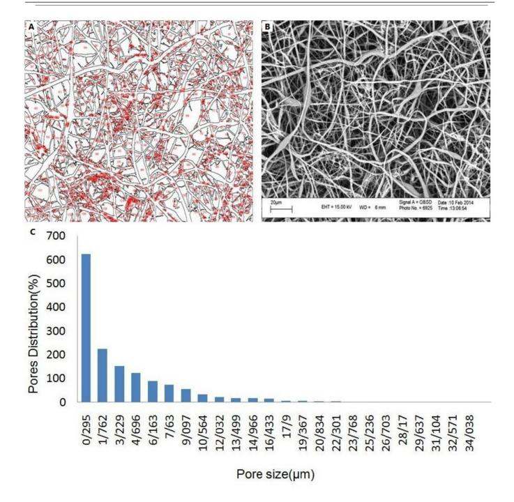
Fig. 2: Image of the distribution of pores in the PCL/nHA Scaffold (A) Graphical image of pore position, (B) SEM image ×3000 (C) Pore distribution diagram
